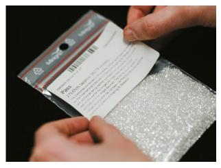
**Figure 2:** Melee screening services are offered by several gemtesting laboratories. The diamonds in this parcel were identified as natural by the International Institute of Diamond Grading & Research. Photo courtesy of De Beers Group Industry Services.
