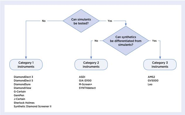
**Figure 5:** This flowchart shows the process for determining a DVI's operational category. The instruments listed were Assure tested as of July 2019. Courtesy of DPA.
